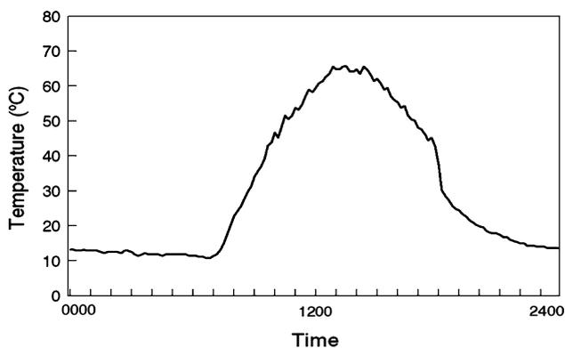
**Fig. 2** Typical diurnal heating curve within closed black plastic bag inside clear film tent (“double tent”). Reference ambient air maximum = 34.1°C (taken from nearby CIMIS weather station, Oakdale, San Joaquin Valley, Station #194). Sept 3, 2010, Oakdale, CA
